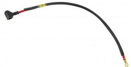
Alternator wiring loom Diesel engines 8.1985 and later
