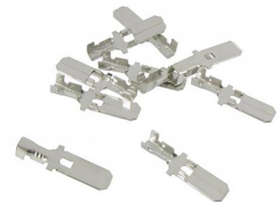
Uninsulated male spade connectors without locking barb (10 pieces) Spade connector size: 6.3mm, Material thickness: 0.8mm, Wire thickness: 1.5 - 2.5mm 2
