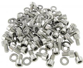
Stainless steel shroud screws including washers (50 pieces) Thread size: M6 x 1.0, Length: 10mm, Material: stainless steel A2, Tensile load: 70, Wrench size: 5mm, Washer diameter: 11.70mm
