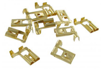
Uninsulated right angled female spade connectors with locking barb (10 pieces) Spade connector size: 8.0mm, Material thickness: 0.8mm, Wire thickness: 1.5- 2.5mm 2
