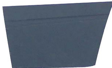
Door repair panel left Vanagon/T25
