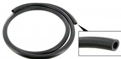
Oil hose textile braided per meter inner Ø 12.7 outer Ø 20.0mm
