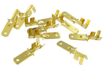
Uninsulated male spade connectors with locking barb (10 pieces) Spade connector size: 6.3mm, Material thickness: 0.8mm, Wire thickness: 4.0 - 6.0mm 2
