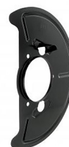
Disc brake splash shield right Vanagon/T25 6.1986 (VIN 2-- G-120001) and later except Syncro
