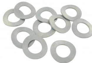
Curved M12 spring washers (10 pieces) Inner diameter: 13mm, Outer diameter: 24mm, Thickness: 1.2mm, Material: Galvanized steel
