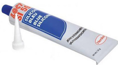
SI 5926 blue silicone sealing compound Content: 40 ml, Color: blue, Chemical Type: Acetoxy Silicone, Maximum sealing gap: 1.0mm, Temperature range: -54 °C to +150 °C
