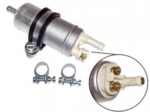
Electric fuel pump A-quality 12V, 0.27 - 0.38 bar, 90 l/h
