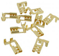
Uninsulated right angled female spade connectors without locking barb (10 pieces) Spade connector size: 6.3mm, Material thickness: 0.8mm, Wire thickness: 1.0-2.5mm 2
