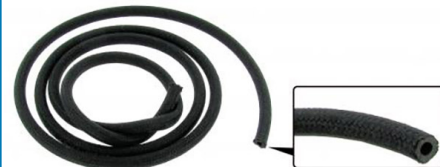
Vacuum hose with a textile outside per meter Inner diameter: 3.5mm, Outer diameter: 7.5mm, Working pressure: 7 bar, Bursting pressure: 30 bar
