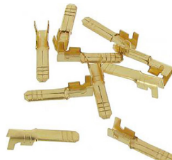
Uninsulated male spade connectors without locking barb (10 pieces) Spade connector size: 2.8mm, Material thickness: 0.8mm, Wire thickness: 0.5 - 1.5mm 2
