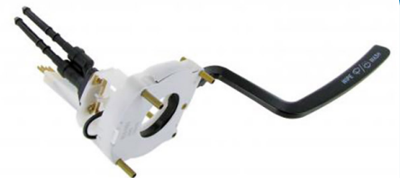
Wiper switch with pneumatic window washer Beetle VW1300, VW1500 and 1302 8.1971 until 1973 (VIN 114 2358 021), 1303 until 1973 (VIN 134 2358 021), Karmann Ghia, 8.1971 and later, Type 3, 8.1971 and later, Thing 3.1973 until 1974 (VIN 184 2356 315)
