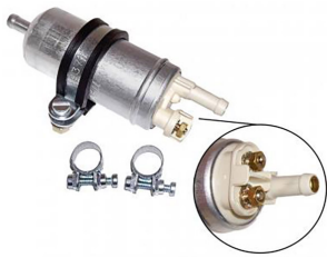
Electric fuel pump A-quality 12V, 0.27 - 0.38 bar, 90 l/h
