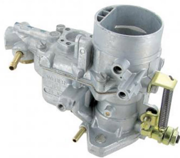
Weber 34 ICT carburetor (each) Main jet: 135, Air jet: 160, Idle jet: 55, Emulsion tube: F78
