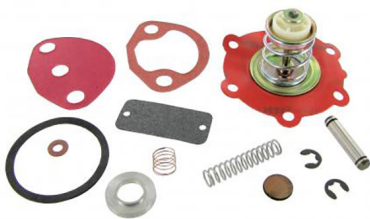
Fuel pump rebuild kit Type-1 engine 1200cc (34hp) until 7.1965, Type-3 engine until 7.1965
