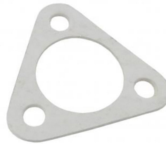
Header to muffler gasket (each) Bolt distance: 58mm, Inner size: 44.70mm
