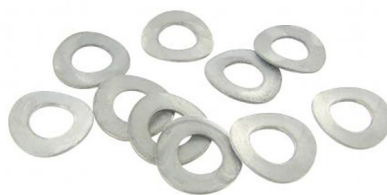
Curved M10 spring washers (10 pieces) Inner diameter: 10.5mm, Outer diameter: 21mm, Thickness: 1.0mm, Material: Galvanized steel
