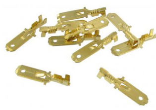
Uninsulated male spade connectors with locking barb (10 pieces) Spade connector size: 6.3mm, Material thickness: 0.8mm, Wire thickness: 0.5 - 1.0mm 2
