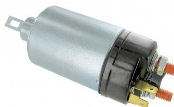
Starter solenoid 12V Beetle 8.1969 and later, Karmann Ghia 8.1969 and later, Bus with an aircooled engine 8.1966 and later, Type 3 8.1969 and later
