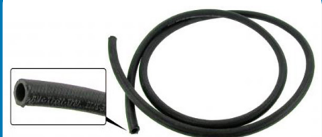
Breather hose with a textile outside per meter Inner diameter: 12mm, Outer diameter: 17mm, Working pressure: 7 bar, Bursting pressure: 30 bar
