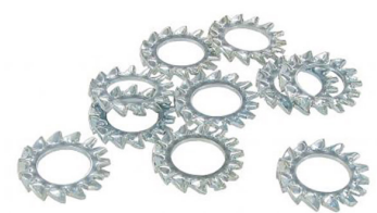
External serrated lock washers M8 (10 pieces) Inner diameter: 8,4mm, Outer diameter: 15mm, Height: 2.4mm, Material: Galvanized steel
