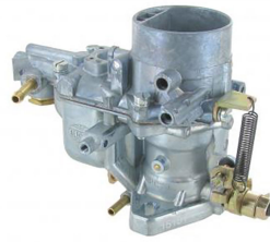
EMPI EPC 34 Carburetor (each) Main jet: 150, Air jet: 175, Idle jet: 55, Emulsion tube: F6
