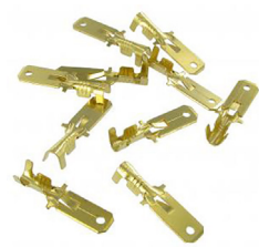
Uninsulated male spade connectors with locking barb (10 pieces) Spade connector size: 6.3mm, Material thickness: 0.8mm, Wire thickness: 1.5 - 2.5mm 2
