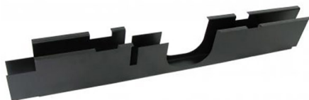
Rear crossmember brace overlap panel Bus 8.1967 until 7.1979
