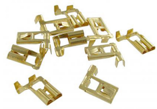
Uninsulated right angled female spade connectors with locking barb (10 pieces) Spade connector size: 8.0mm, Material thickness: 0.8mm, Wire thickness: 1.5- 2.5mm 2
